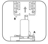
Step 2. Make sure LIFELIGHT adaptor insert direction is correct. Adaptor orientation key(A) is positioned opposite to track key(B)\*. Or align with recessed track slot for adaptor orientation key to sit in.
